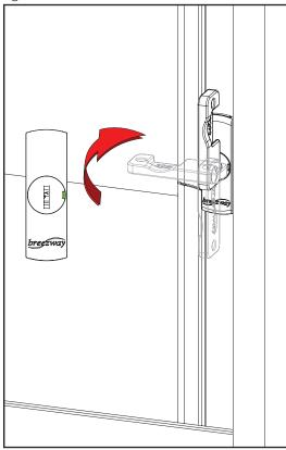
Rotate key into unlocked position, note green unlocked indicator on barrel face when in the unlocked position as shown in Figure 5.
