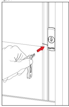
Remove key to secure locking barrel in place. Lock is not secured until key is removed from barrel as shown in Figure 3. Window is now locked.
