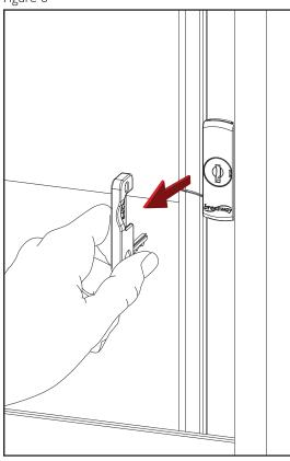
Remove key after barrel is rotated into unlocked position, the window is now unlocked.
